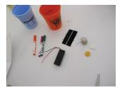
Materials: toy motor, AA battery and case, 2 plastic cups, 3 markers, double-sided tape, offset motor weight (yellow), velcro
