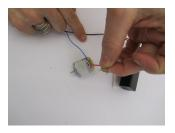
2) Take one red wire from the motor and one red wire from the battery pack and cross the ends
