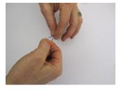
1) Carefully twist the metal ends of each of the two wires attached to the motor. This will bunch the wires together so they do not fray.
