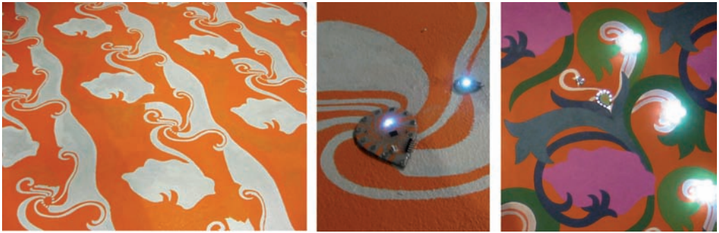
Fig. 13. Living Wall. (left) The circuitry layer (in silver) being painted. (center) Magnetically attached microcontroller and LED modules on the unfinished surface. (right) A completed flower pattern with a microcontroller, two lamps, and a proximity sensor.
