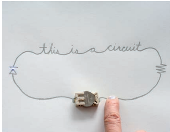
Fig. 16. A painting of a circuit, a schematic diagram, and a functioning circuit.
