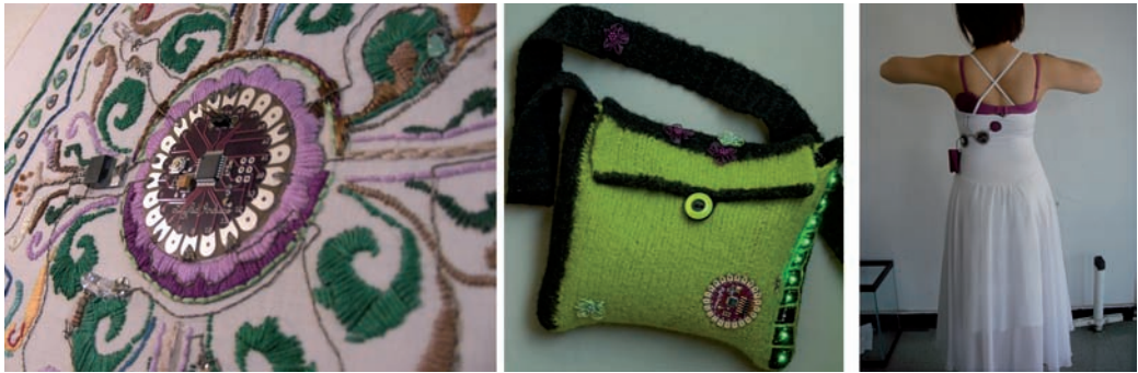
Fig. 14. Three projects built by LilyPad Arduino adopters, from left to right: interactive embroidery, a handbag that stores and plays back knitting patterns, a dance costume that tracks its wearer's movements and communicates with other costumes.
