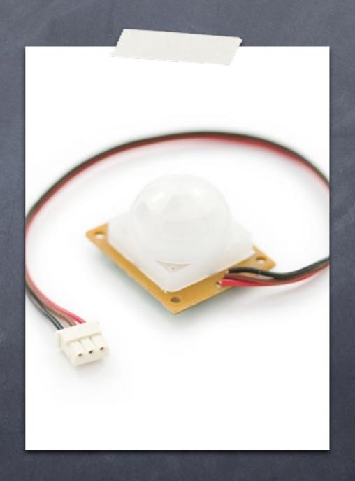
This unit works great from 5 to 12V (datasheet shows 12V). You can also install a jumper wire past the 5V regulator on board to make this unit work at 3.3V. Sensor uses 1.6mA@3.3V.
