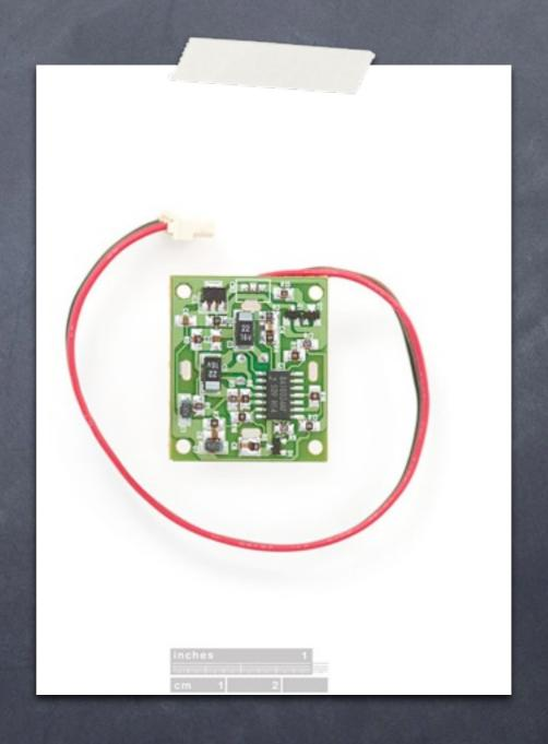
Note: The colors of the wires can vary greatly. Looking at the unit from the top, the middle wire is ground, the left-most wire is the alarm, and the right-most is the power.
