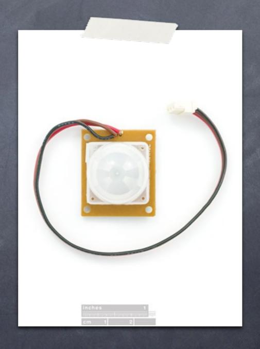
The alarm pin is an open collector meaning you will need a pull up resistor on the alarm pin. The open drain setup allows multiple motion sensors to be connected on a single input pin. If any of the motion sensors go off, the input pin will be pulled low.
